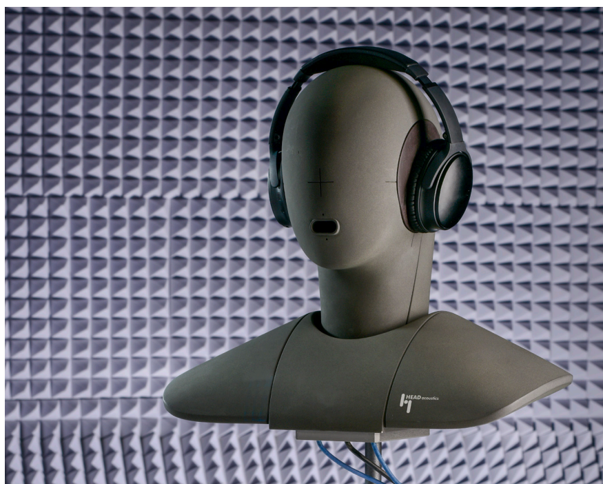
Exemplary measurement setup for EN50332 compliance of a Bluetooth headset on HMS II.3.
