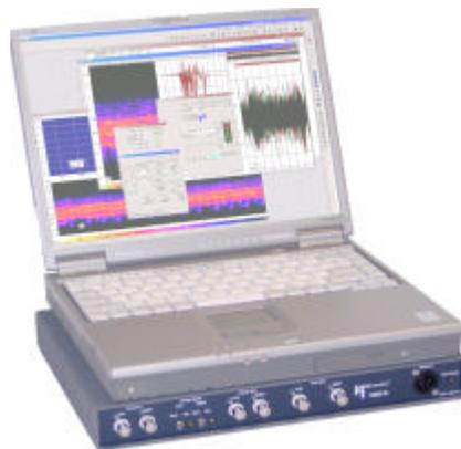
Standard pulse sensors can be directly connected to the Supply Box. HSB IV is fitted with an internal pulse conditioning and extraction component. Four-channel recordings (executed via two Artificial Heads) are also no problem for HSB IV.
