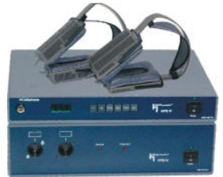
The entire system provides aurally-accurate conditioning of Artificial Head recordings, enabling authentic, true-to-original playback of sound events. PVA IV.3 is equally appropriate for A/B comparisons, professional audio applications, or for playback of conventional recordings.
