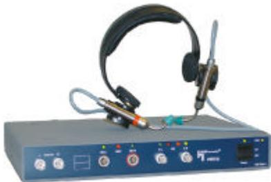
Built-in rechargeable batteries make BEQ II independent-of-mains for a number of hours. Via the AES output featured in BEQ II you are also able to execute recordings using a DAT recorder.
