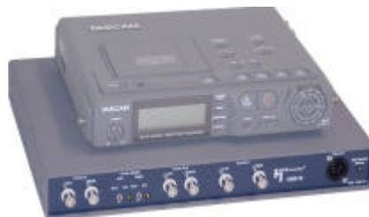
Measurement data can be recorded via a DAT recorder or a notebook. All parameters and functions of the Artificial Head, the DAT recorder and the notebook can be selected, modified and executed by connecting the RC V remote control.
